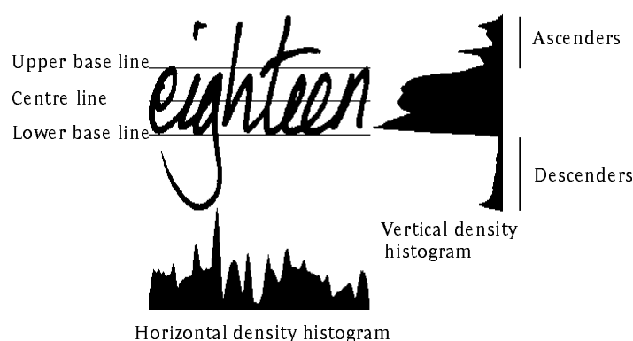
Figure 5.2: Histograms, centre line and base lines.
