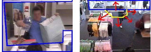
Figure 5: Views from the customer service desk (left) and a door (right). The “region of uninterest” in which detections are ignored to reduce false positives is outlined in blue. Alert tripwires ( enter and leave ) are drawn on the door view.
